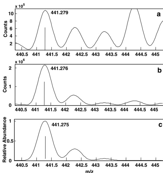
**Figure 6.** (a) Rejected peak at  $m/z$  441.279 from the verapamil incubate spiked with a bile matrix. (b) Retained peak with monoisotopic  $MH^+$  ion at  $m/z$  441.276 from verapamil incubate spiked with a bile matrix. (c) Theoretical mass spectrum of demethylated verapamil with monoisotopic  $MH^+$  ion at  $m/z$  444.275.
