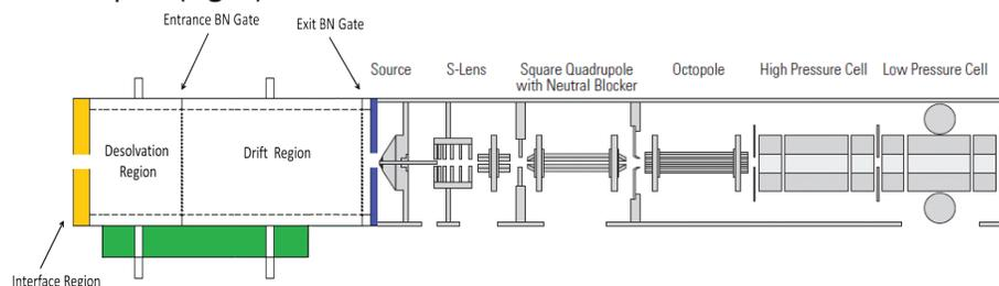
**Figure 2.** Representation of the dual gate ion mobility module interfaced with a Thermo Scientific™ LTQ Orbitrap Velos™ mass spectrometer indicating ionization interface region (shown with no source), desolvation region, ion gate #1, drift region, ion gate #2, and focusing lens of the IMS-MS interface.
