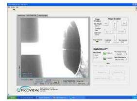
PV Acquire v2.0.0 software package which accompanies the Digital PicoView system. The automated Digital Divert mode is active, as shown in the image.
