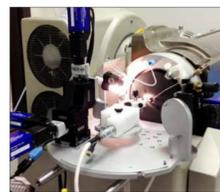
Digital PicoView DPV-450 nanospray source installed on an AB SCIEX 4000 Q TRAP instrument.
