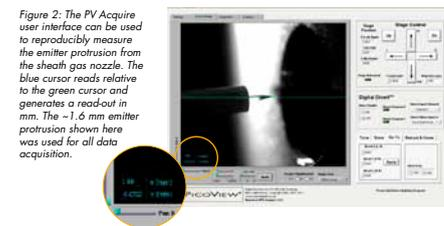
Figure 2: The PV Acquire user interface can be used to reproducibly measure the emitter protrusion from the sheath gas nozzle. The blue cursor reads relative to the green cursor and generates a read-out in mm. The ~1.6 mm emitter protrusion shown here was used for all data acquisition.
