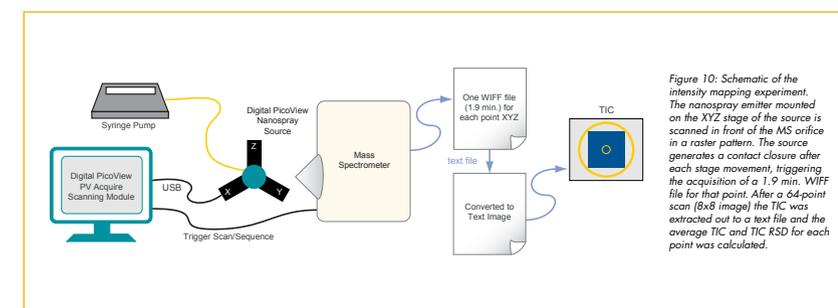
Figure 10: Schematic of the intensity mapping experiment. The nanospray emitter mounted on the XYZ stage of the source is scanned in front of the MS orifice in a raster pattern. The source generates a contact closure after each stage movement, triggering the acquisition of a 1.9 min. WIFF file for that point. After a 64-point scan (8x8 image) the TIC was extracted out to a text file and the average TIC and TIC RSD for each point was calculated.
