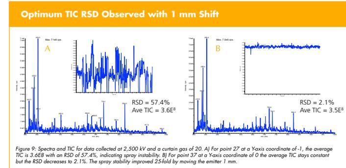
Figure 9: Spectra and TIC for data collected at 2,500 kV and a curtain gas of 20. A) For point 27 at a Y-axis coordinate of -1, the average TIC is 3.6E8 with an RSD of 57.4%, indicating spray instability. B) For point 37 at a Y-axis coordinate of 0 the average TIC stays constant but the RSD decreases to 2.1%. The spray stability improved 25-fold by moving the emitter 1 mm.
