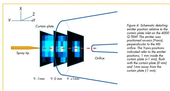
Figure 4: Schematic detailing emitter position relative to the curtain plate inlet on the 4000 Q TRAP. The emitter was positioned on-axis (Y-axis), perpendicular to the MS orifice. The Y-axis positions indicated refer to the emitter positions: 1 mm inside the curtain plate (+1 mm), flush with the curtain plate (0 mm) and 1 mm away from the curtain plate (-1 mm).
