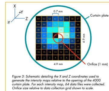
Figure 3: Schematic detailing the X and Z coordinates used to generate the intensity maps relative to the opening of the 4000 curtain plate. For each intensity map, 64 data files were collected. Orifice size relative to data collection grid shown to scale.
