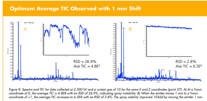
Figure 8: Spectra and TIC for data collected at 2,500 kV and a curtain gas of 10 for the same X and Z coordinates (point 37). A) At a Y-axis coordinate of 0, the average TIC is 4.8E8 with an RSD of 26.9%, indicating spray instability. B) When the emitter moves 1 mm to a Y-axis coordinate of +1, the average TIC increases to 6.5E8 with an RSD of 2.8%. The spray stability improved 10-fold by moving the emitter 1 mm.
