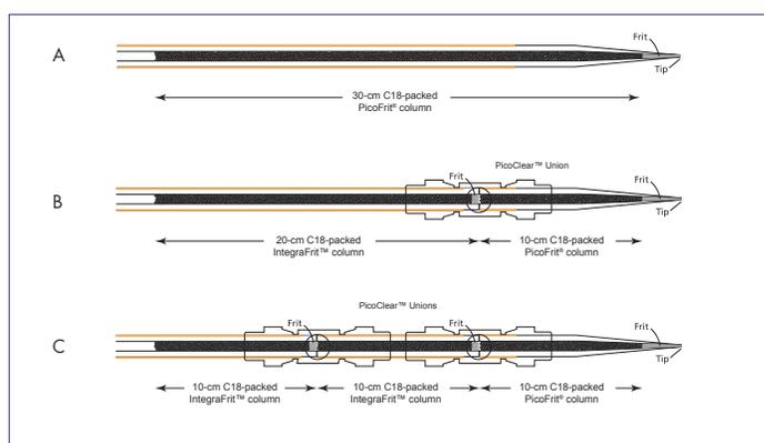
**Figure 4** Schematic diagrams of PicoClear union-column combinations. A) PicoFrit column with 30 cm bed, B) 20 cm IntegraFrit coupled to a 10 cm PicoFrit column with a PicoClear Union, and C) Two 10 cm IntegraFrit columns coupled to a 10 cm PicoFrit column via two PicoClear Unions
