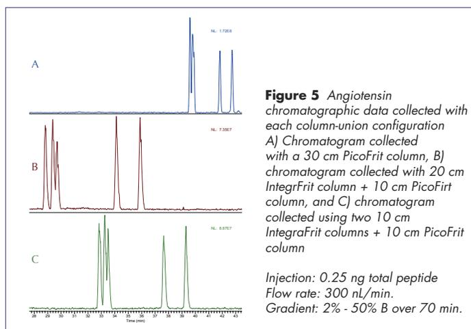
**Figure 5** Angiotensin chromatographic data collected with each column-union configuration A) Chromatogram collected with a 30 cm PicoFrit column, B) chromatogram collected with 20 cm IntegraFrit column + 10 cm PicoFrit column, and C) chromatogram collected using two 10 cm IntegraFrit columns + 10 cm PicoFrit column
