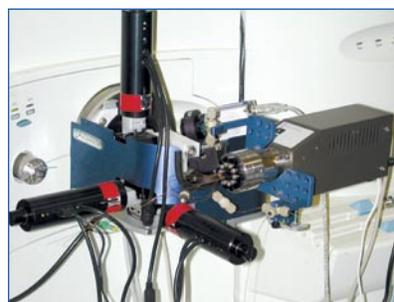
**Figure 3** Digital PicoView® nanospray source on LCQ Deca™ mass spectrometer
