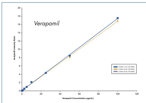
**Figure 6** Linear dynamic range behavior of verapamil using three tip IDs
