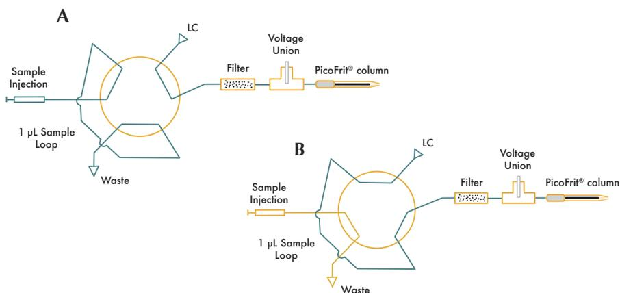
A standard 6-port injection scheme (1 µL volume) was used with in-line filtration (1 µm porosity) to preserve column integrity. ESI high voltage was applied pre-column directly to the mobile phase through a platinum wire micro-electrode. Pre-column volume was kept to a minimum ( $\leq 1 \mu\text{L}$ ) to minimize the gradient delay.
